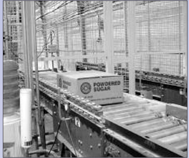
▲ Boxes are filled with bags of sugar and moved along an assembly line where they are loaded onto pallets for shipment.
